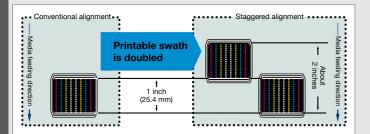
Improved ink jetting angle achieves higher print image quality without grainy appearance in 4-colour mode by jetting variable size dots, Large, Medium and Small variable dots, with a maximum resolution of 1440dpi
