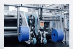
The **delivery section** incorporates pneumatically adjustable pressure zones for a wide range of folding carton styles and an adjustable belt speed for different shingle modes.
