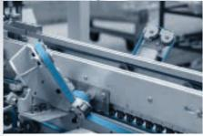
The long **pre-folding section** achieves 180° folding on creasing line 1 and 135° on creasing line 3 as well as many possibilities to implement folding elements.
