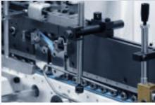
The modular **lock bottom section** includes a servo-driven back folding system, allowing the FB II Bestfold to adapt flexibly to specific customer requirements.
