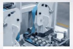
Adjustable **folding belts** maintain consistent accuracy and eliminate misalignments, ensuring flawless results even at high speeds.
