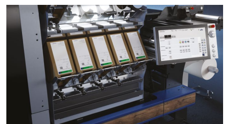
Optimised ink management: The redesigned ink management system with operator access speeds up and simplifies replacement of ink containers without any risk of contamination.
