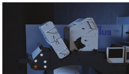
Automatic splice detection: The Gallus One automatically detects splices, letting them pass all print bars without loss of register and speed.
