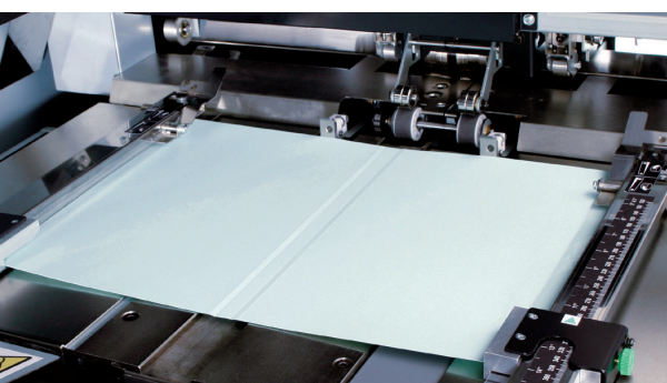
Covers are automatically scored and presented onto the nipping table
