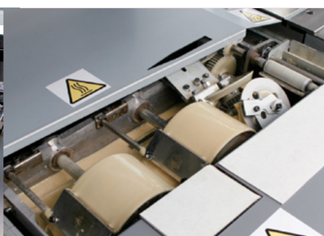
Glue drums with automatic side gluing and glue cut off control
